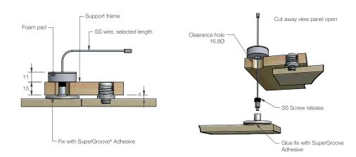
Seismic restraint providing added security and control. The panel is suspended below the ceiling for convenient servicing behind the panel or controlled removal of the panel by releasing the wire.
