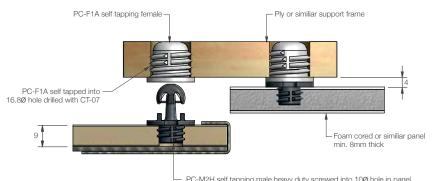
PC-M2H self tapping male heavy duty screwed into 100 hole in panel
