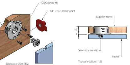
The Fastmount autofit PC-AF1 is ideal for applications that require lateral adjustment, such as curved panels. This versatile screw-fixed clip works with all Standard range male clip types.
